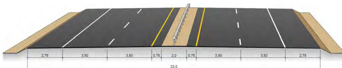
Figur 2-1 Normalprofil for H3 (handbok N100, 2021).
